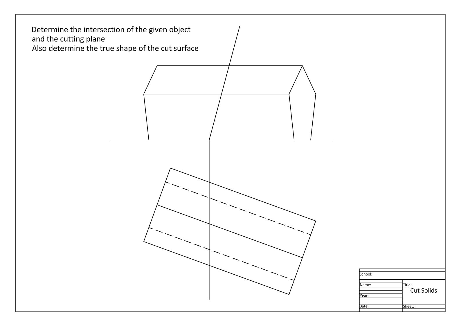
Determine the intersection of the given object and the cutting plane Also determine the true shape of the cut surface
