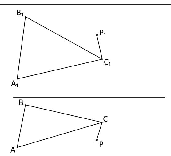
Find the true inclination of the line PC to the Lamina ABC
